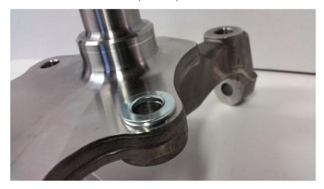
2. Next orient your bracket so the largest hole is centered over the upper mount on the spindle and using the 1½ long ½ bolt capture the M12 washer between the bracket and spindle.
