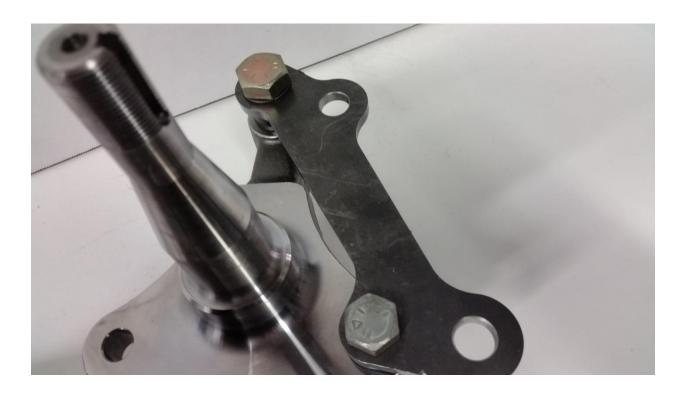
5. Tighten your bolts sung to allow no movement for mock up and assemble the hub to the spindle
